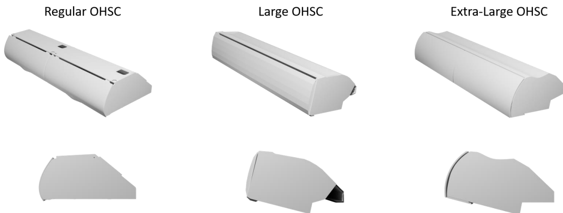
Figure 9. Graphical representation of the three overhead stowage compartment variants.
