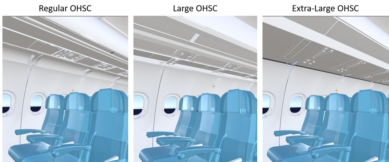
Figure 11. Visualization of the hatrack configuration in VR for all variants.
