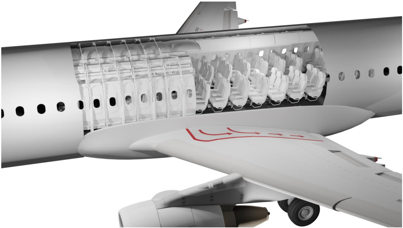
Figure 10. 3D model of the aircraft cabin concept with the extra-large hatrack.
