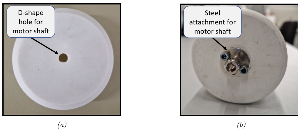
Figure 4.3: Original drum mount (a); New drum mount with steel coupling (b)
