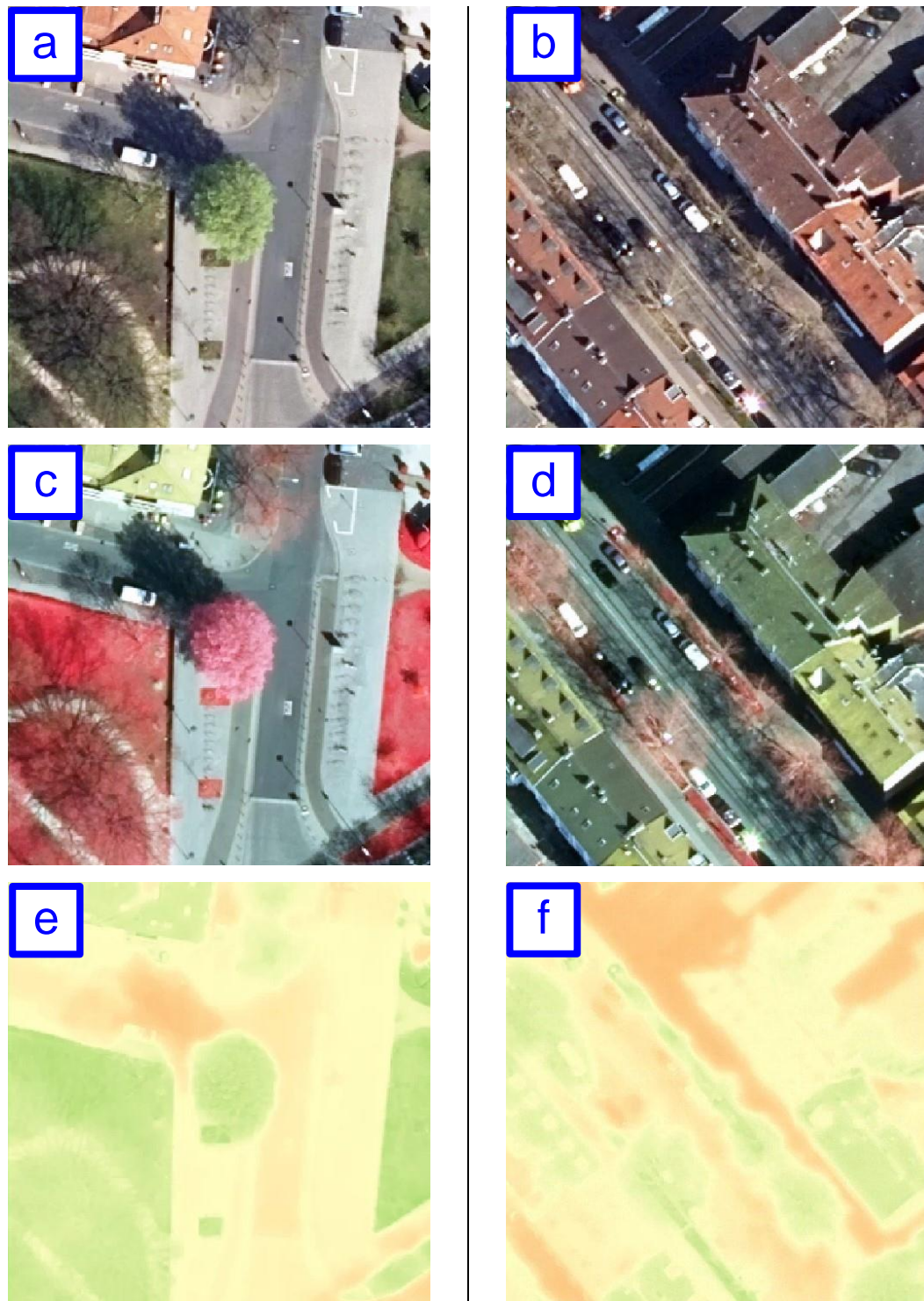
Figure 5. Healthy tree (left) and non-healthy tree (right) with natural color band combination (a,b), CIR band combination (c,d), and NDVI (e,f). Source: Landesamt für Geoinformation und Landesvermessung Niedersachsen - LGLN (2022).
