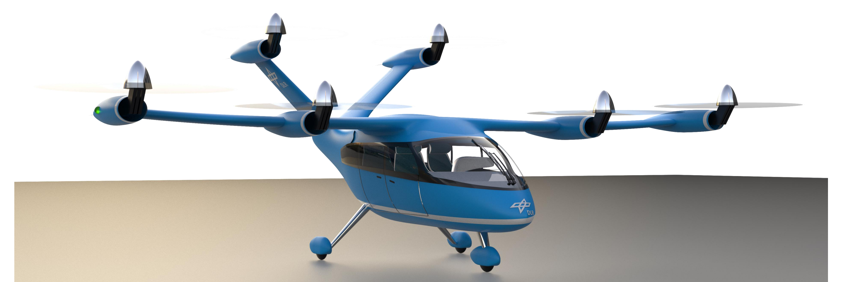
Tiltrotor vehicle concept based on optimal top level aircraft requirements. Credits: DLR.
