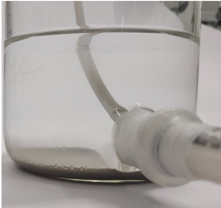
Figure 5.17: Visible Layer of Lunar Regolith Simulant after 24 Hours during Sedimentation Experiment
