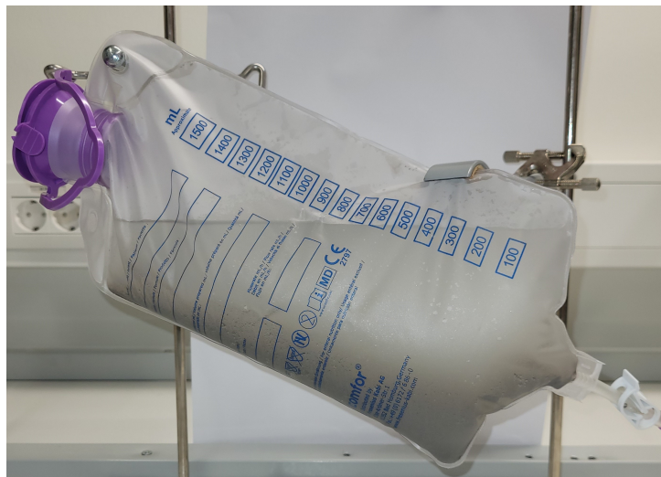
Figure 5.5: Structure of Sedimentation Experiment Using Infusion Bag
