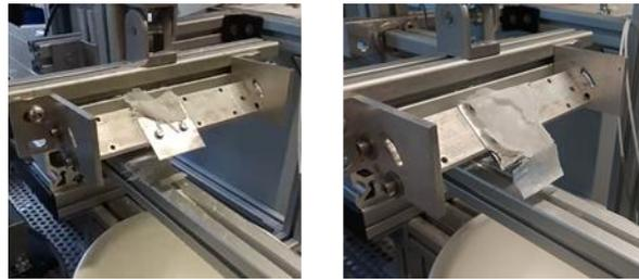
Figure 4: Picture of scraped PCM. Left: Decanoic acid. Right: Paraffin.
