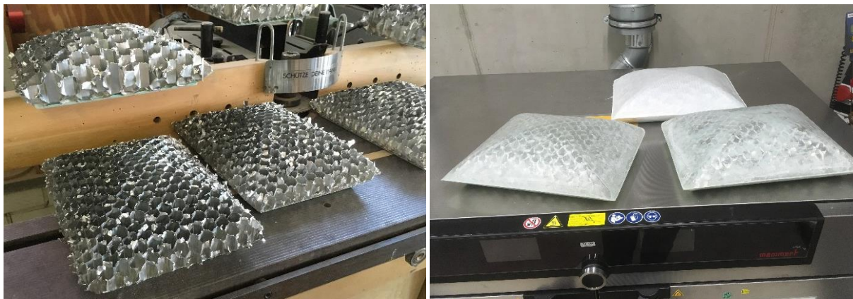
Fig. 3-6: Comparison of aluminum honeycomb cushion after contour milling (left) and after face-sheet lamination (right).
