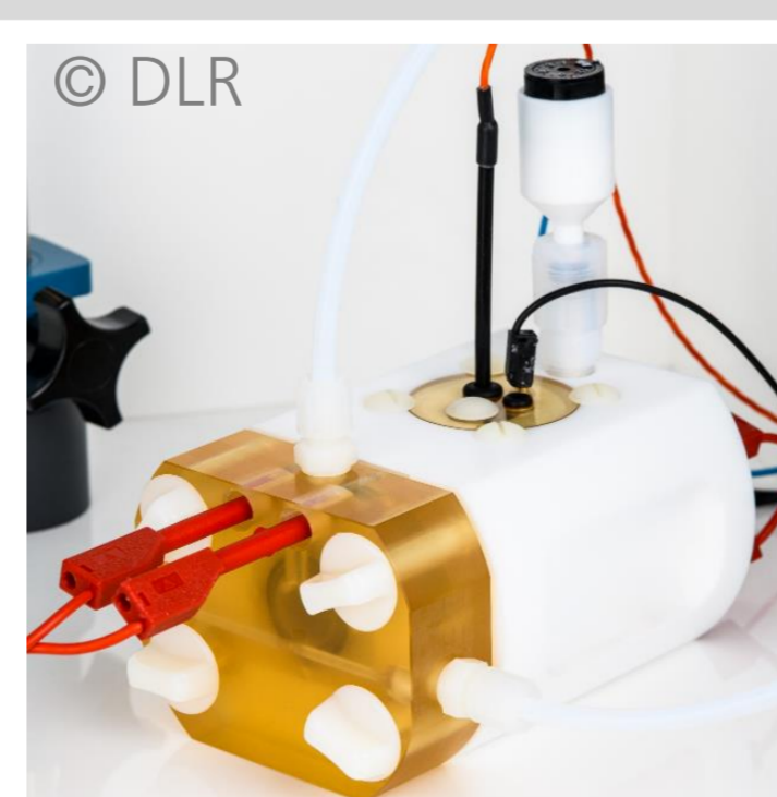
Fig. 6. Commercial GDE half-cell setup (Gaskatel FlexCell PTFE®)
