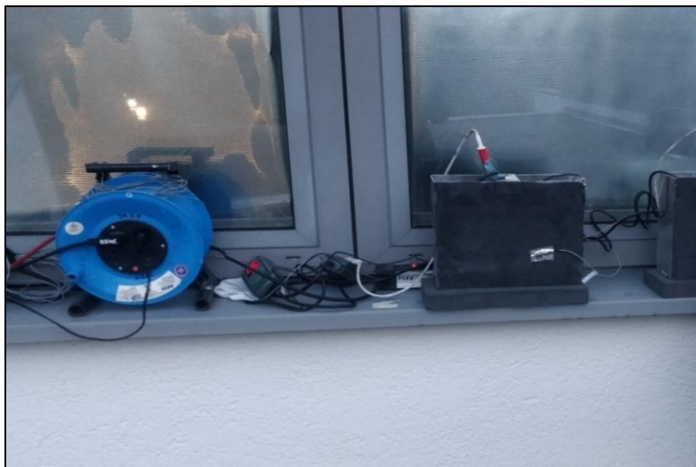
Figure 15. Reference body with temperature control and surface temperature measurement.
