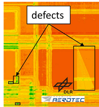
Fig. 2. Sample NDT data with defects (magnified).
