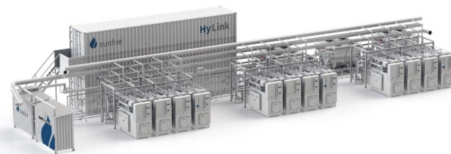
Figure 7. Sunfire SOEC-HyLink system [131] (graphics with permission from Sunfire).
