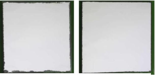
Sample after 2 years exposure in Almeria: coastal site, corrosion class C5 after ISO 9223
