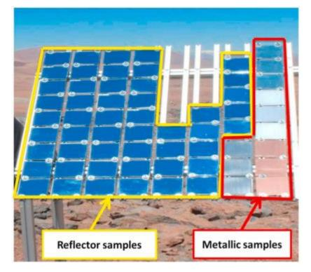
Reflector and standard metal samples in outdoor exposure rack.
