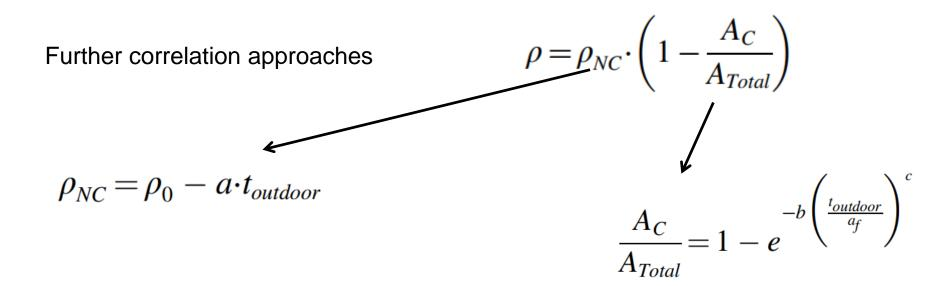
Non corroded area shows linear degradation of reflectance, due to erosion, UV-degradation or soiling deposition
