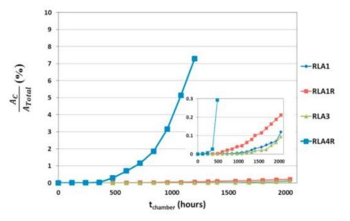
Find testing time in CASS to reproduce same corrosion area as after 3 years outdoor.
