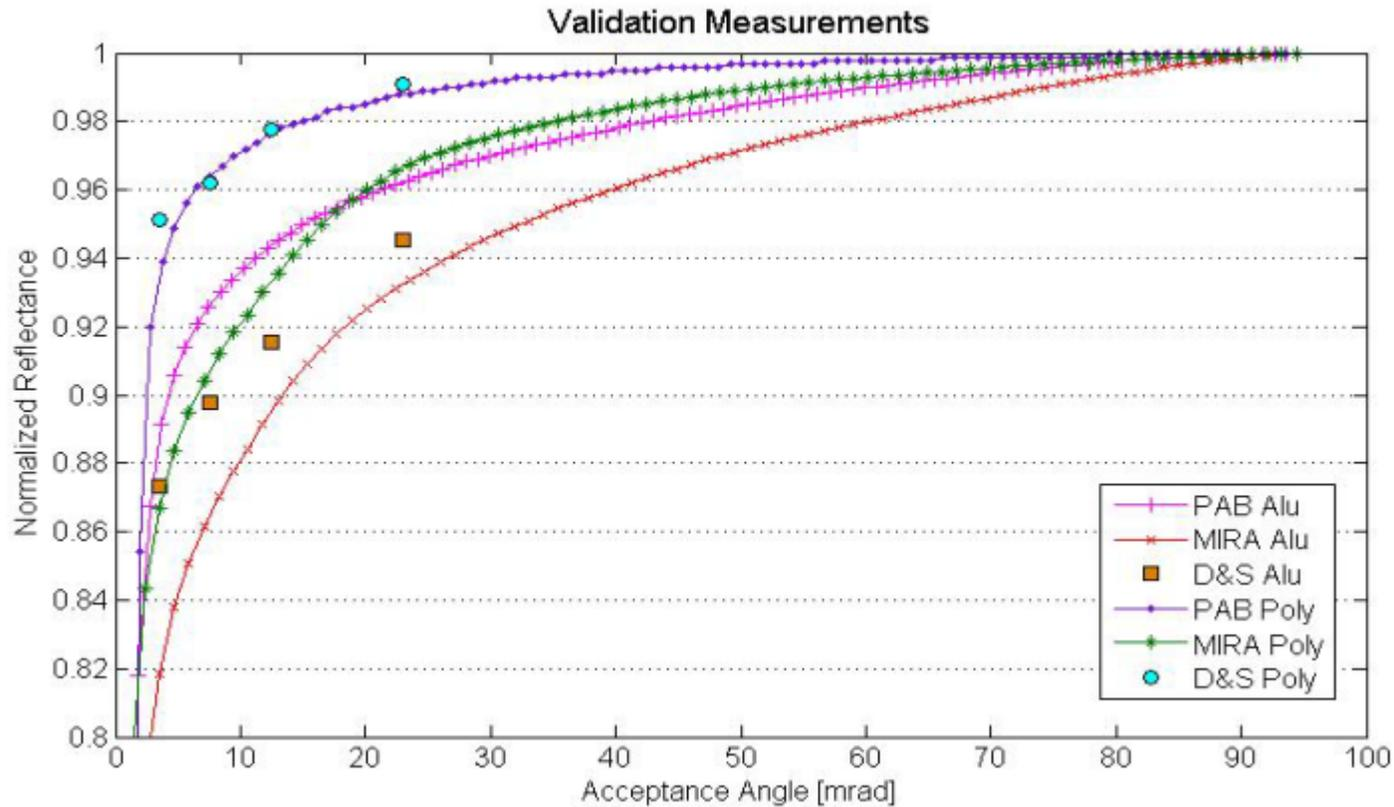
D&S measurements at slightly different wavelength
