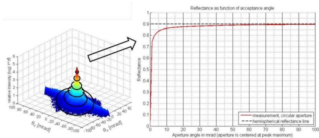
Backscattered Reflectance Distribution Function can be spherically integrated to Reflectance Over Acceptance angle function
