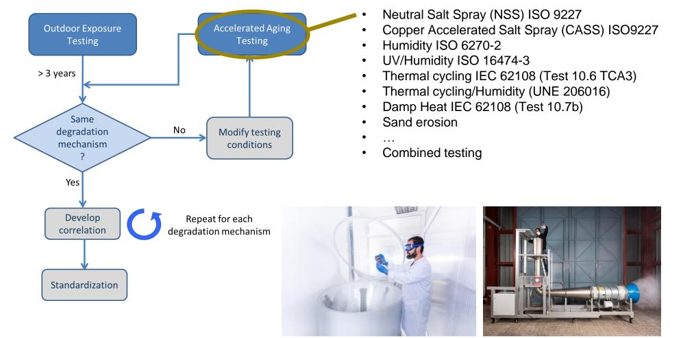
Salt Spray testing according to ISO 9227 Sand erosion test bench at PSA
