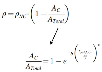
Acceleration factor  $a_f$ derived from comparison of CASS test with outdoor results.
