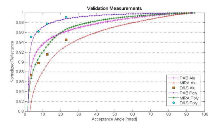
D&S measurements at slightly different wavelength
