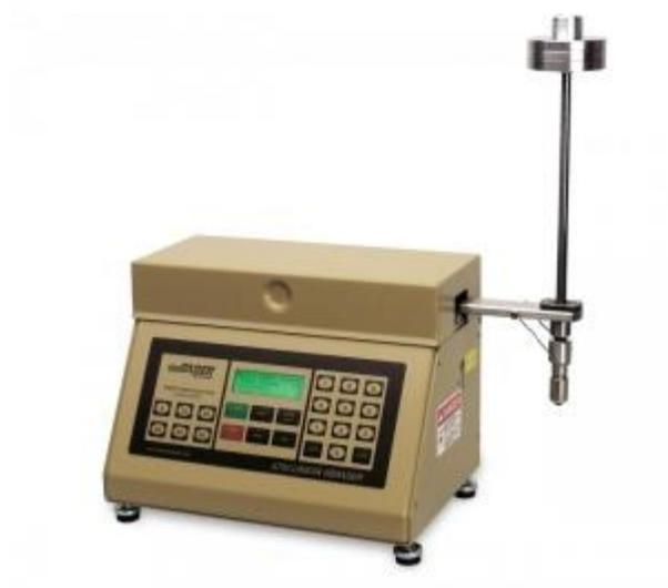
Scratching of coatings with controlled normal force
