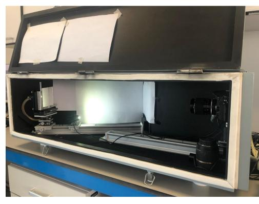
10 x 10 cm<sup>2</sup> sample results in ca. 5000 x 5000 pixel area.  $\rightarrow$  1 pixel = 20µm
