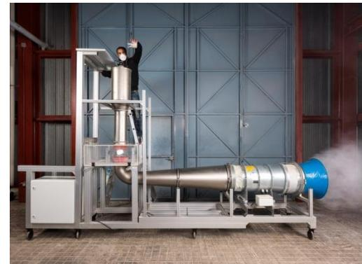
Sand erosion test bench at PSA
