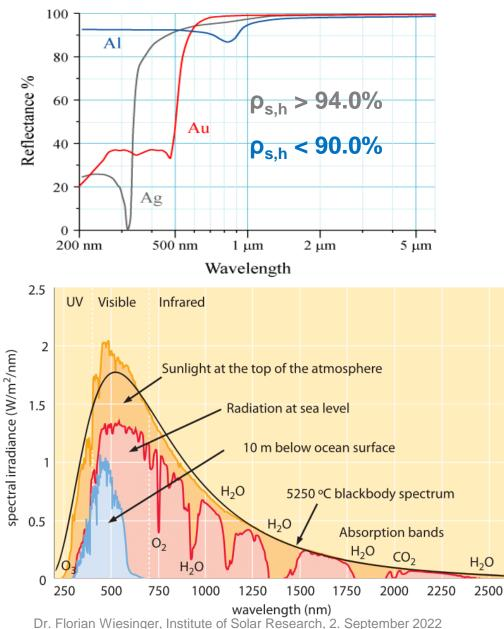
A suitable "mean value" of all relevant solar wavelengths is the solar weighted reflectance
