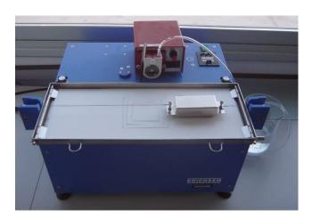
Simulation of cleaning cycles
