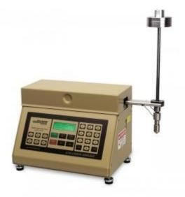
Scratching of coatings with controlled normal force
