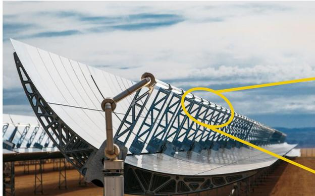
Parabolic trough collector
