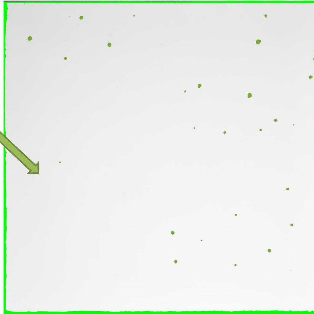
Divide Aged image (AI) by Reference Image (RI) and detect every pixel with less than certain brightness ratio of initial brightness as corrosion.
