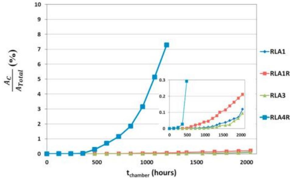
Find testing time in CASS to reproduce same corrosion area as after 3 years outdoor.
