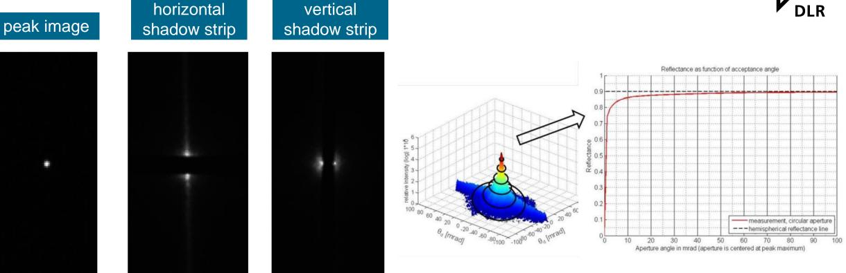
Backscattered Reflectance Distribution Function can be spherically integrated to Reflectance Over Acceptance angle function
