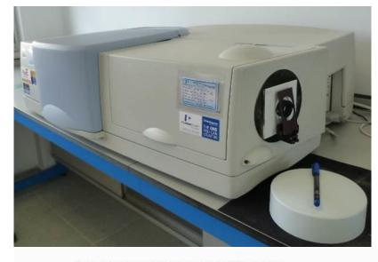
Spectrometer with 150mm Integrating Sphere
