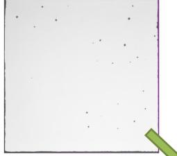
Divide Aged image (AI) by Reference Image (RI) and detect every pixel with less than certain brightness ratio of initial brightness as corrosion.
