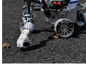
(b) View of the back side of LRU2 showing the Jaco2 arm with a robotic hand attachment performing a stone collection task. The rc-visard camera attached to the back provides visual feedback during manipulation.
