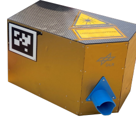
Figure 4: The LIBS payload box with nozzle for constant distance between rock and spectrometer.
