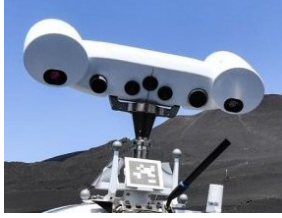
(a) Large pan-tilt unit of LRU which includes a stereo camera pair for depth perception as well as spectral imaging cameras to gather additional information about the geological makeup of potential samples found in the environment
