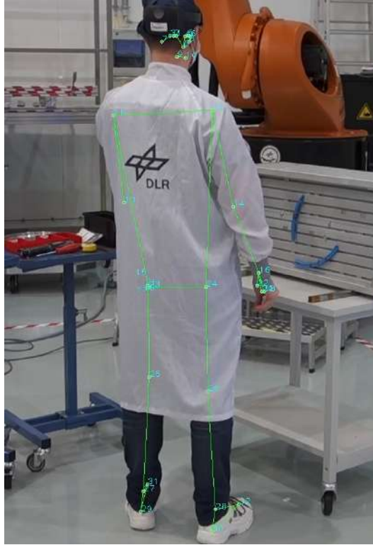
Figure 4.23.: An example frame showing the landmarks detected by the PoseEstimation software
