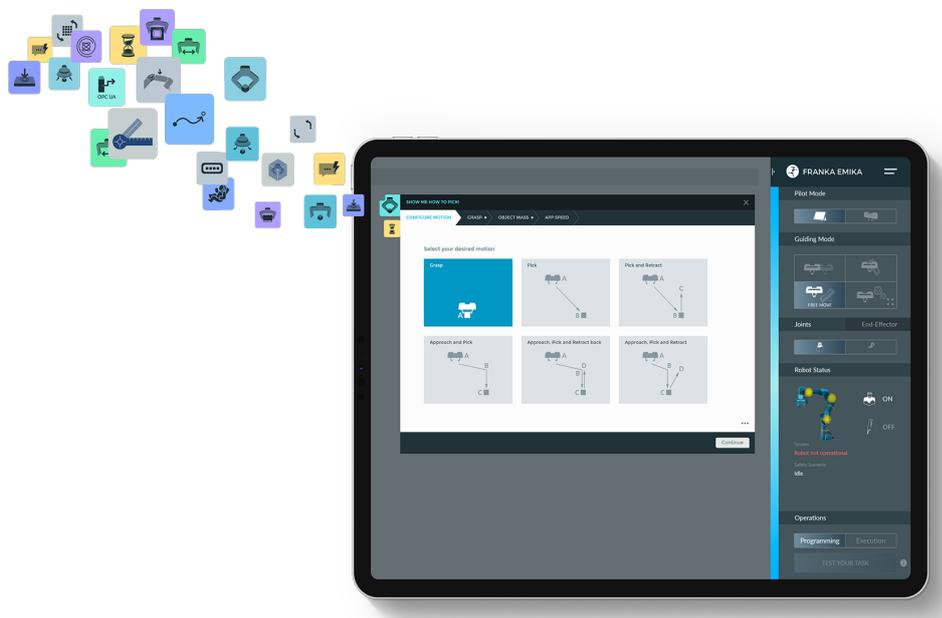
Figure 2.3: The GUI used for FRANKA EMIKA products, that utilizes a workflow-based robot programming approach [EMI].
