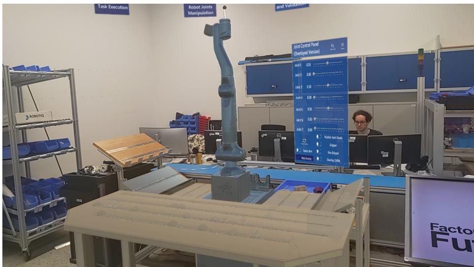
Figure 3.29: The overlaid workbench and SARA robot on top of the real one.
