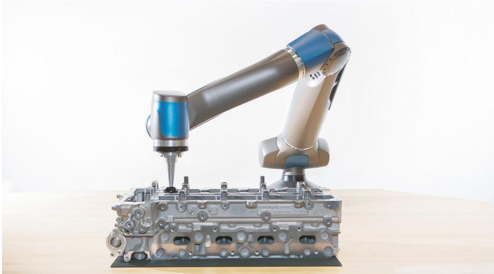
Figure 3.5: The DLR's new generation of lightweight robots, SARA, developed at the Center of Robotics and Mechatronics (RMC) [SAR].
