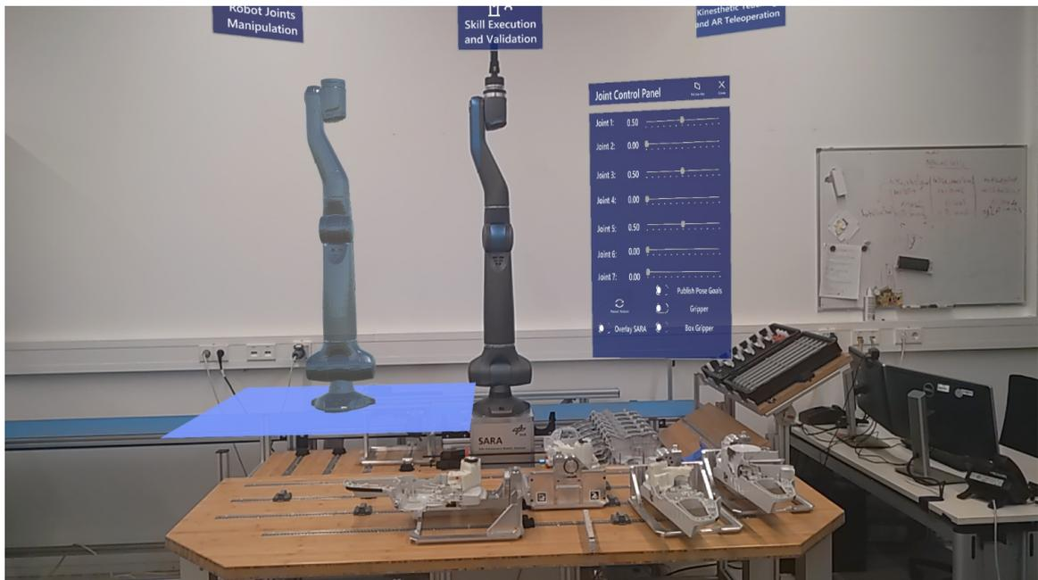
Figure 3.18: The "Robot Joint Manipulation" module that enables individual joint configuration of the robot.
