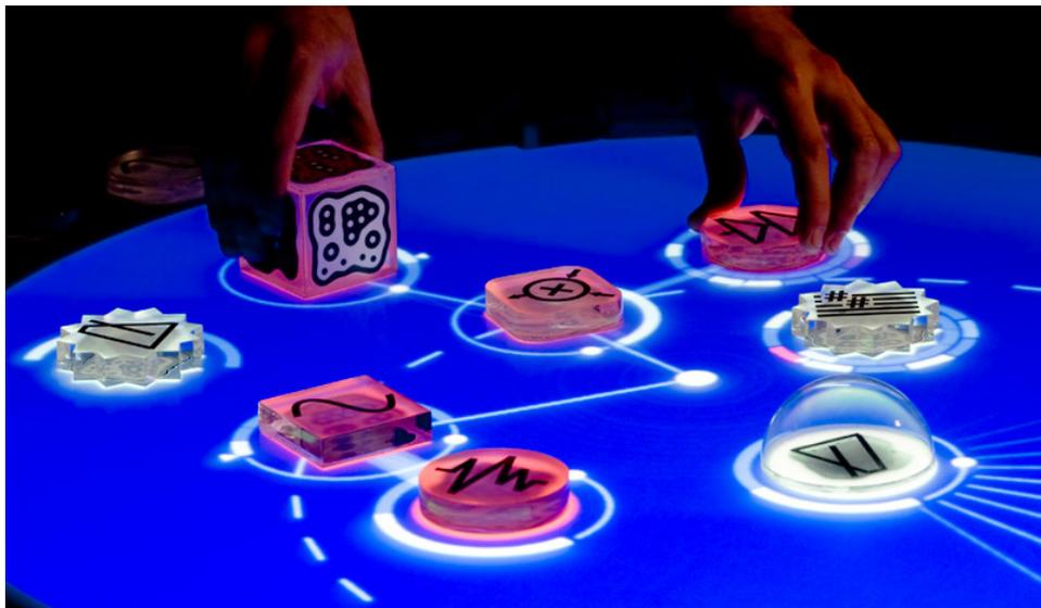
Figure 2.4: Tangible User Interface on a projected table [vLGG19].
