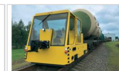
ExpressService ES3000 battery electric shunter (© ExpressService)
