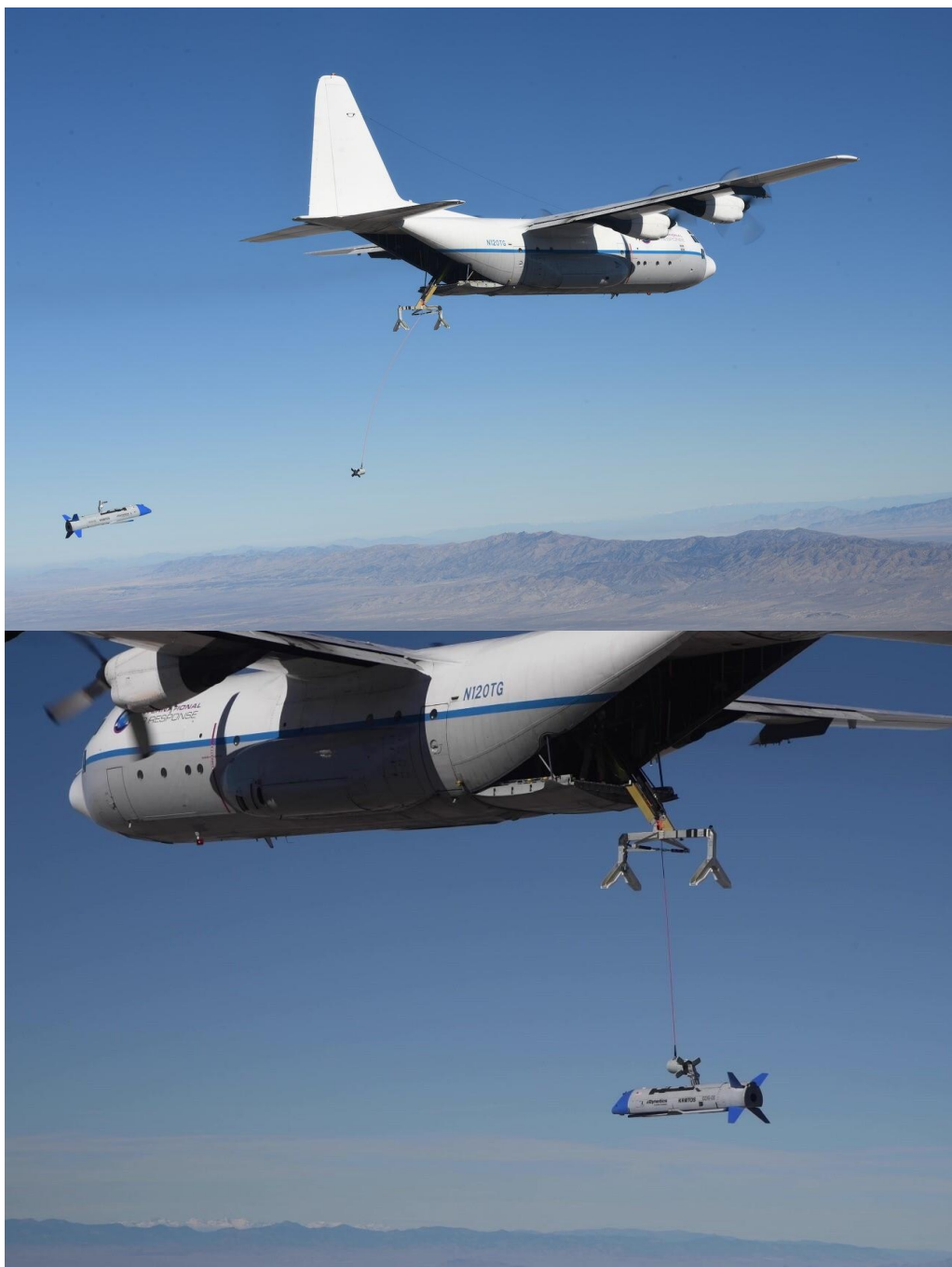
Figure 18: X-61A successful in-flight capturing maneuver (October 2021)
