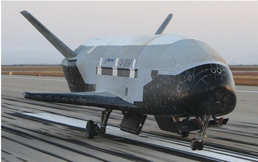
Figure 17: Reusable X-37B with own landing gear assembly and open gear bay doors after landing
