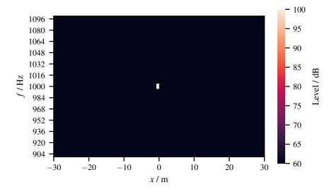
*Figure 5: The results of the deconvolution using the new propagation model. The system matrix of Fig. 3 was used. The frequency range considered in the deconvolution was* 904 Hz to 196 Hz. *The computed level at the center point at* 1000 Hz *is* 99 dB.
