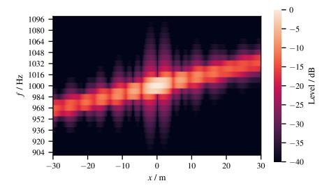
Figure 4: The modeled point spread function of a single virtual source located at the center of the grid, with  $f_s = 1000$  Hz. The values in this plot represent a single column in the system matrix (Fig. 3).
