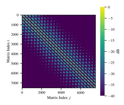
Figure 3: The new system matrix of the deconvolution problem calculated with eq. (25). The setup corresponds to the flyover described by Fig. 1. Each block represents a frequency pair  $f_s$ ,  $f_f$ , with  $f_s = f_f$  on the diagonal. The displayed frequencies range from 904 Hz to 196 Hz.
