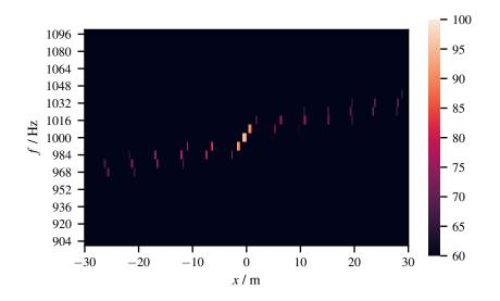
Figure 2: Results of the hybrid deconvolution as described by [6] results of the simulated source of Fig. 1. As this deconvolution does not consider the interconnection of frequencies, it is unable to resolve them and correctly locate the tonal source, both in space and frequency. The amplitude at x = 0 m and f = 1000 Hz is underestimated with 96.2 dB.
