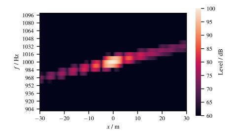
Figure 1: Beamforming results of a monopol at altitude 200 m and  $v_x = 80 \text{ m/s}$ . The source is a tonal source with 1 kHz and 100 dB. The line array consists of 101 equally spaced microphones, For demonstration purposes, the geometric setup replicates the beamforming pattern in [5].
