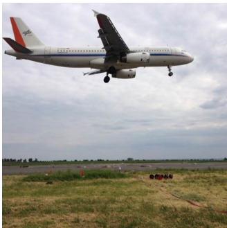
Figure 1: The Aircraft ATRA (A320) has repeatedly been used for flyover measurements with a microphone array [2].
