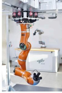
(a) The first demonstrator of the SwarmRail system, with a LWR attached at the bottom of it [36].
