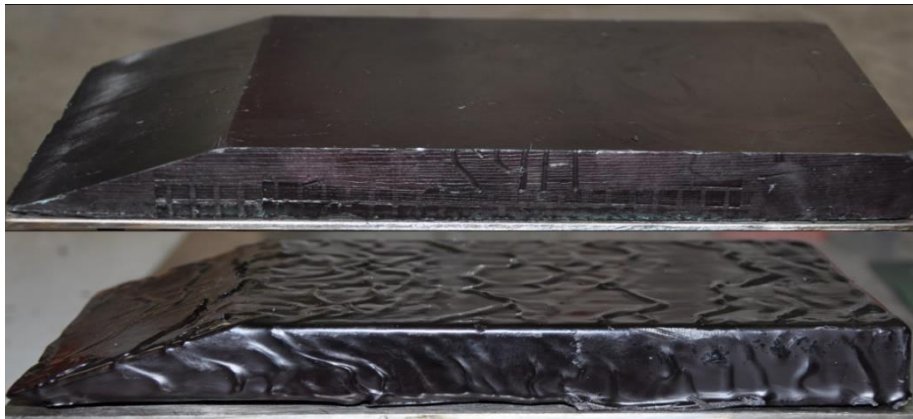
Fig. 1: Fuel slab configuration before (top) and after (bottom) combustion test
