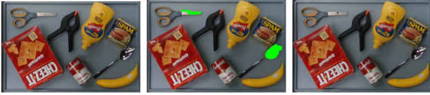
Fig. 8. Magnetic grasp pipeline. The initial RGB image (left) is fed to the segmentation network that provides a mask of the metallic objects, which is double-checked with the depth information to have more accurate masks (center). The centroids of the masks constitute potential magnetic grasps, as depicted in the right image by the points on the scissor and the spoon.
