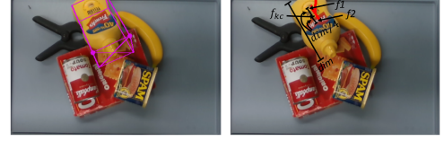
Fig. 7. Fingertip positioning with the double suction single object modality. After the cuboid detection (left figure), being \text{dim} the dimension of the principal axis of the upward face, the fingertips are placed equidistant from the center by a factor of \frac{\text{dim}}{4} to guarantee a stable grasp aligned with the principal axis of the face.
