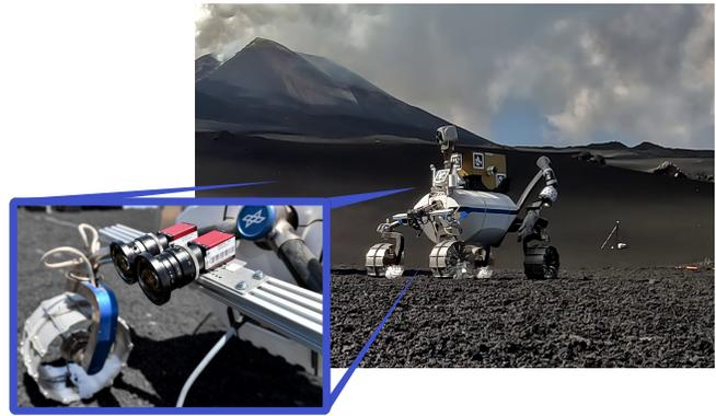
**Figure 9:** SUPER stereo-camera setup, here mounted between the front wheels on the LRU rover at a height similar to the MMX rover. Credits: Felix Oprean, DLR.
