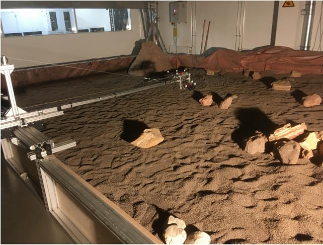
**Figure 10:** View of DLR-RM’s Planetary Exploration Laboratory (PEL). The SUPER camera stack is mounted on a beam that is moved via a linear slide. The ground truth is measured via the ARTrack tracking system using spherical reflective markers. PEL is currently upgraded to a Phobos analog setup.
