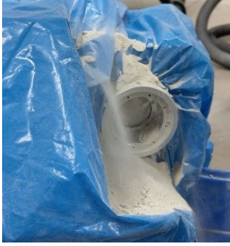
Figure 22. Dust break-in test setup.
