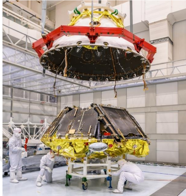
Fig. 5. Planetary Protection measures against contamination by spacecraft, here ExoMars assembled and tested under planetary protection constraints. Credit: ESA ExoMars Program/Thales Alenia Space.
