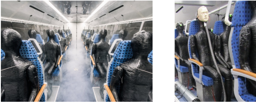
Fig. 1 The generic train compartment equipped with thermal manikins during a smoke visualization (left); with the aerosol-exhalating face and aerosol particle sensors (right) ©DLR.
