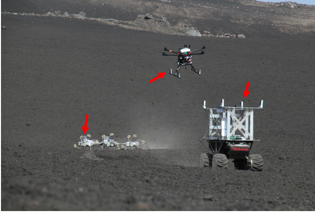
Figure 17: Mission scenario on Mt. Etna robots with attached UWB devices.
