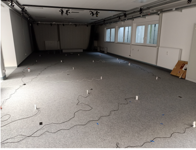
(a) Experimental setup in the holodeck: static nodes are deployed on the ground. The positions of all nodes are tracked by the optical tracking system mounted on the ceiling.
