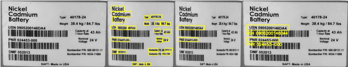
Fig. 4: Type sign image, raw EAST ROI output, refined ROIs, part and serial number from Tesseract OCR (left to right)
