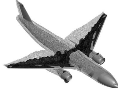
Figure 6. Perspective view of the integration volumes for viscous pressure (grey) and wave drag (black).
