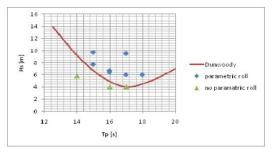
Figure 6. Comparison of test results, line is the calculated result, the markers are experimental, Hs is the significant wave height and  $T_P$  the wave peak period, for a container vessel of 250 meters lengths.
