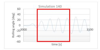
Figure 12. Strong parametric rolling with  $v_s$ = 7,25kn,  $\beta$  = 0°,  $T_w$ =17,87s,  $\lambda$ = 382m, H=17,88m
