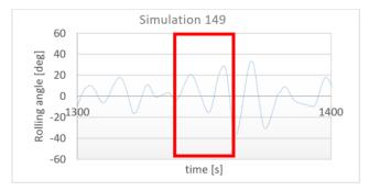
Figure 10. Very extreme parametric rolling with  $v_s$ = 7,25kn,  $\beta$  = 0°,  $T_w$ =17,87s,  $\lambda$ = 382m, H=23,84m
