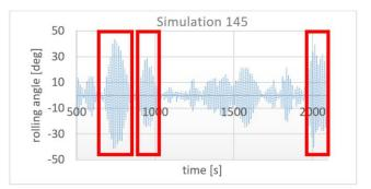
Figure 9. Serial parametric rolling with  $v_s$ = 7,25kn,  $\beta$  = 0°,  $T_w$ =17,87s,  $\lambda$ = 382m, H=19,07m
