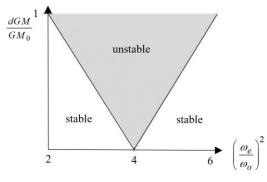
Figure 2. Variation of the metacentric height GM, with the initial metacentric height  $GM_0$
