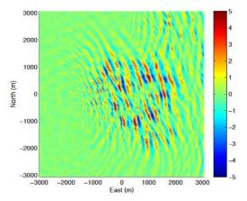
Figure 7. Prediction of T+180s of the wave field, the colors indicate the wave elevation in meters, with a wave direction towards north-east over 3 kilometers.
