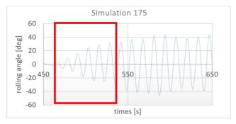
Figure 13. Simple parametric rolling with  $v_s$ = 7,25kn,  $\beta$ = 0°,  $T_w$ =17,87s,  $\lambda$ = 267,4m, H=11,92m
