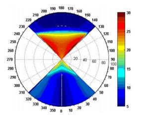
Figure 5. Polar diagram of predicted roll motion, for headings from 0-45 degrees and 135-180 degrees. The warm colors show the areas which exceed 20 degrees of rolling angle. Under the limits, the colors are cold. Vessel speed is from 0-16 knots, the wave height is given with 6 meters and the ratio between ship lengths and wavelength is 1.4. The simulations took each 1200 seconds.
