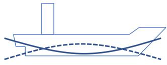
Figure 1. Wave trough and crest.
