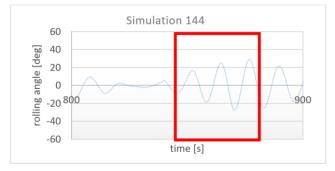
Figure 11. Extreme parametric rolling with  $v_s$ = 7,25kn,  $\beta$  = 0°,  $T_w$ =17,87s,  $\lambda$ = 382m, H=17,88m
