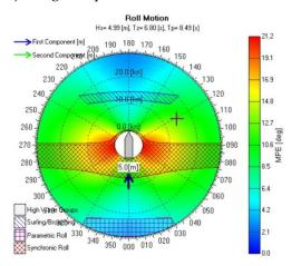
Figure 4. Polar diagram generated by Octopus Software for the sea state  $H_s$ =4,99m (significant wave height),  $T_z$ =6,80s (zero crossing period) and  $T_p$ =8,49s (modal period). The radius shows the ship speed, the colors show the dangerous zones, the headings from 0° to 360° are outlines around, MPE = most probalbe extreme in degree.
