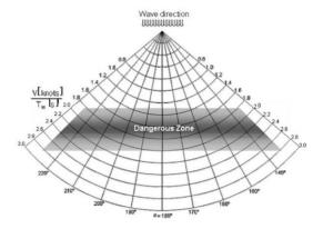
Figure 3. Dangerous zones of synchronous and parametric rolling motions, v is the vessel speed in knots,  $T_{w}$ , the wave period in seconds,  $\alpha$  is the encounter angle, whereby 180° are following seas.
