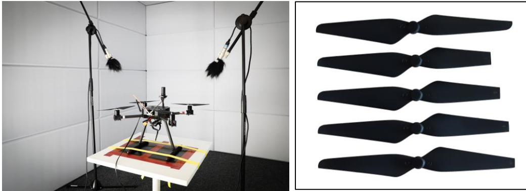
Figure 1. Set-up for data acquisition inside a semi-anechoic chamber (left) and image of propellers used for the recordings (right). From top to bottom: undamaged, 30mm, 20mm, 10mm, and 5mm cut.
