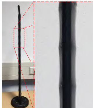
Figure 1 : Side view of the TU Delft Pazy wing with detail of the sagging skin between ribs
