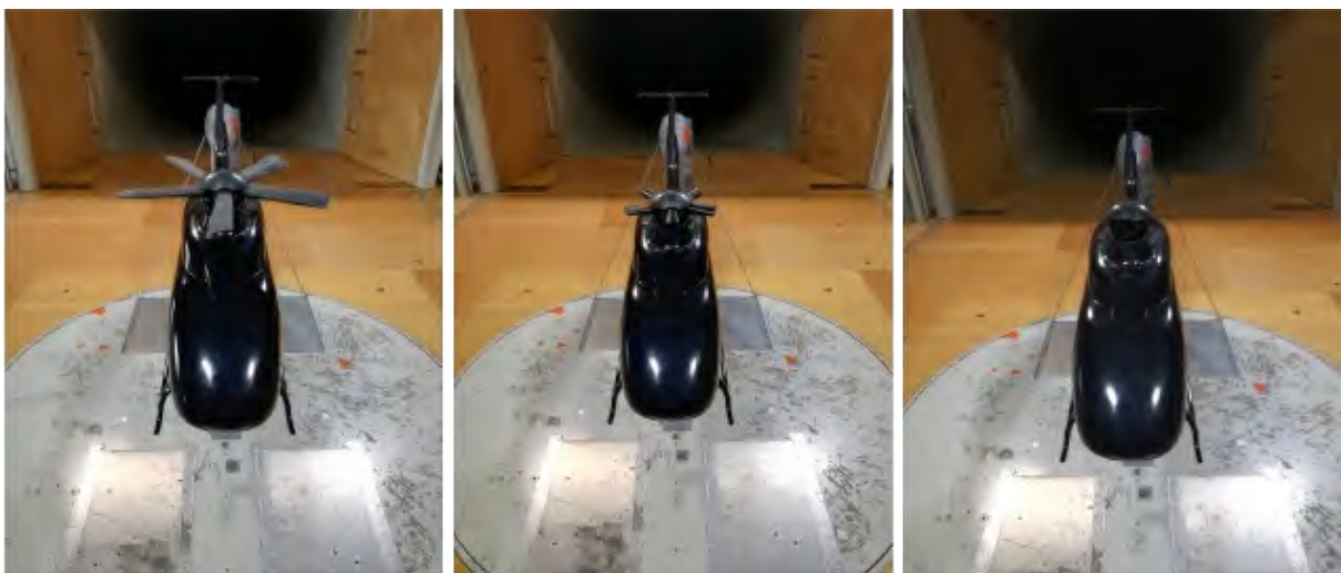
Figure 1: Blade stubs on the helicopter model (left: R1, middle: R2 and right: R3).
