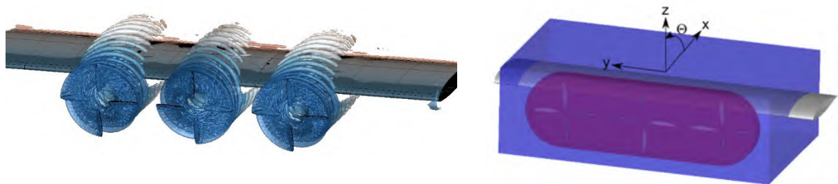
Figure 1 – Vortices visualization by \lambda_2 – value (left) and integration surfaces (right) to obtain acoustic interaction phenomena (blue FW-H 1 and red FW-H 2)
