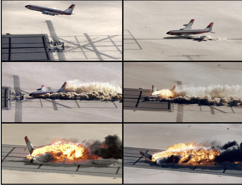
Figure 2.1: Sequence of the Controlled Impact Demonstration (CID) test of a Boeing B720, from [34]
