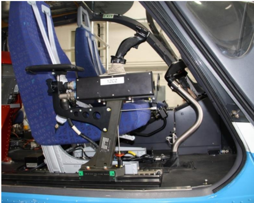
Figure 3-11: Stirling Dynamics Right Sidestick Fitted in DLR EC135 ACT/FHS (source: DLR)
