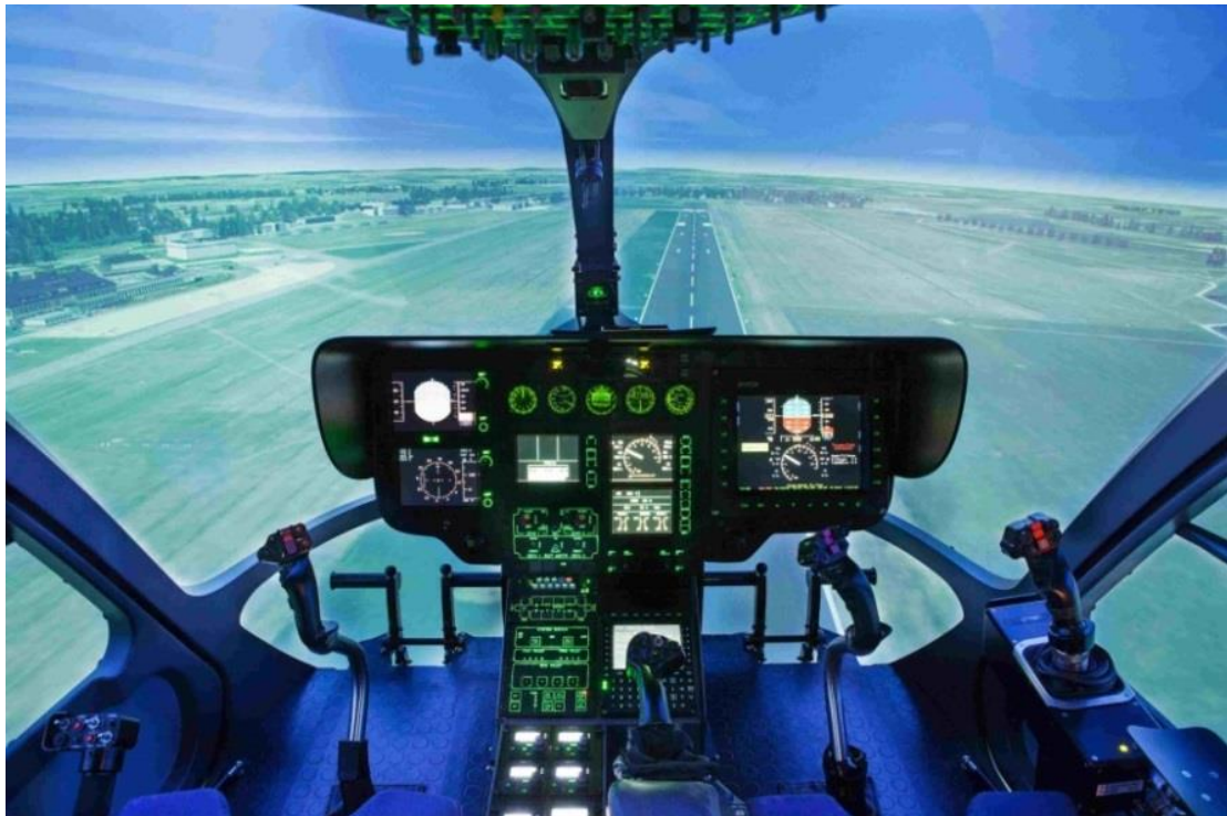
Figure 3-2: Internal View of AVES EC135 ACT/FHS Cockpit, Left and Right Sidesticks Visible at Experimental Pilot (Right) Seat Position (source: DLR)
