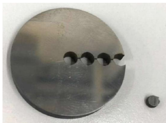
Figure S1: Samples taken to determine the austenite and martensite phase fractions at different radii in the unstrained sample.
