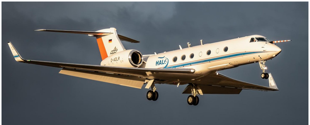
Figure 8: The DLR research aircraft HALO at the landing approach over Edmonton. The protruding stalks on the roof are the trace gas inlets (TGI), the foremost of which is the one used to supply the MIRACLE instrument.
