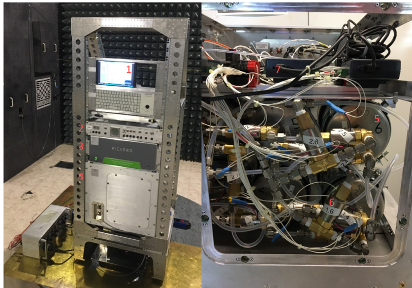
Figure 18: The left part of the picture shows the complete MIRACLE rack at the electro-magnetic interference test laboratory, with the mission monitor(1), the power supply with computer (2), the Picarro analyzer (3) and the sampler box (4). On the right, the stainless steel tanks (5) and the solenoid valves (6) are shown, mounted in the box. The measuring cards, the mass flow controller, the pressure sensors and the pressure relief valve are installed on the intermediate level (7).
