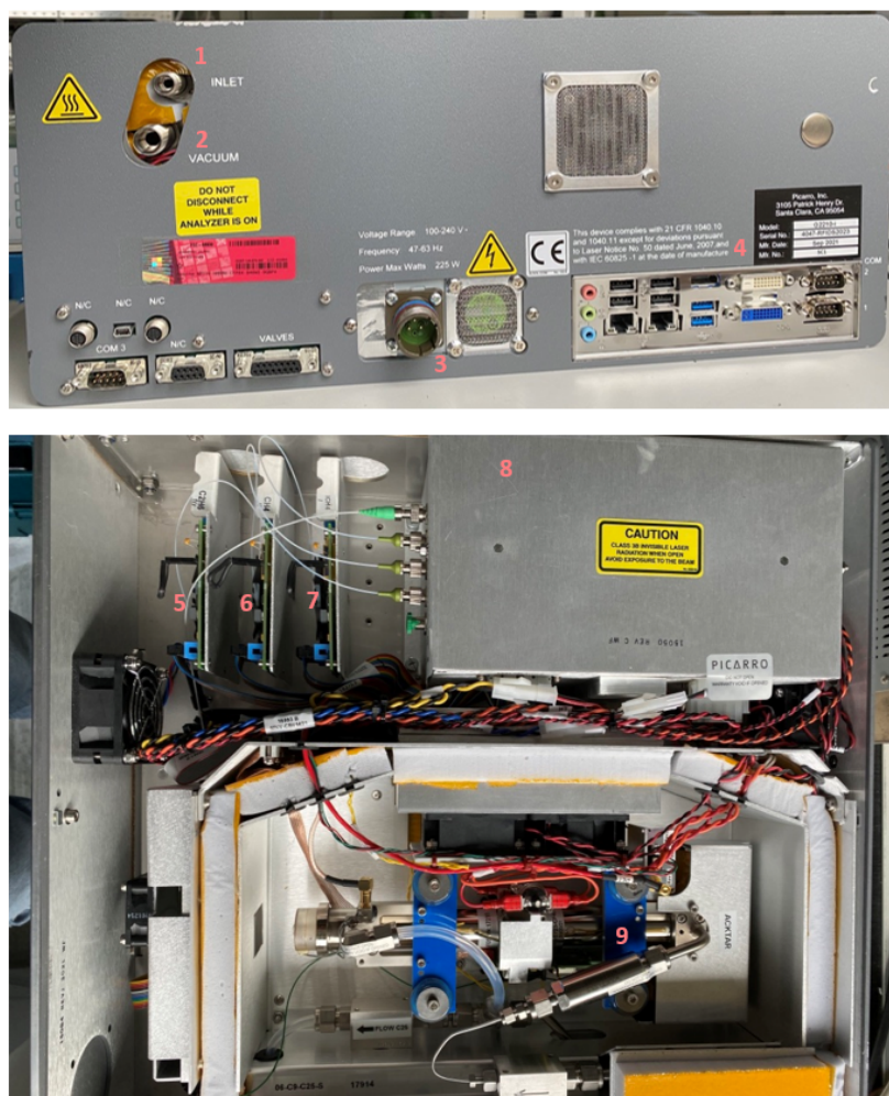
Figure 11: Back view (top) and inside view (bottom) of the Picarro G2210-i greenhouse gas analyser. The numbers indicating the individual components.
