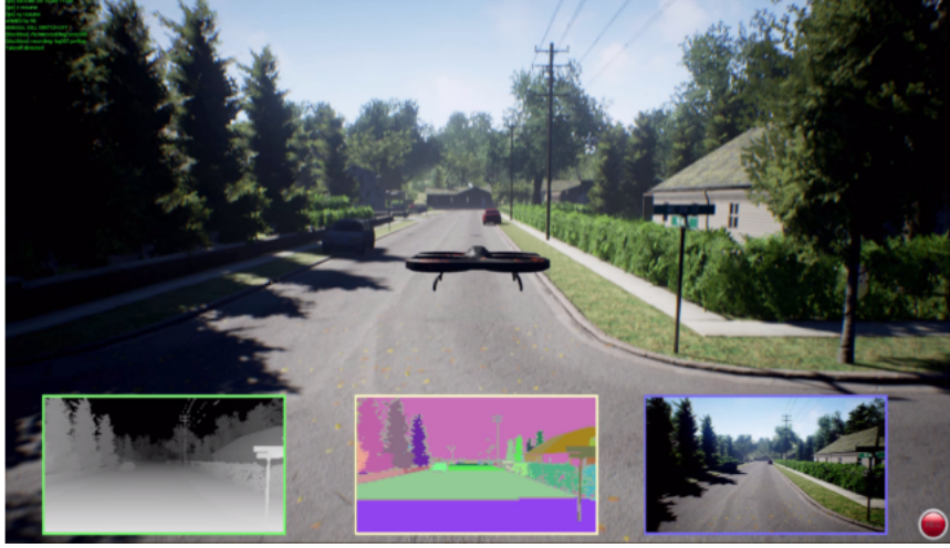
Figure 3.1: A snapshot from AirSim shows an urban environment in which a UAV is flying. The depth image stream, the materials property view stream and the front camera image stream are shown in real time in the inset.
