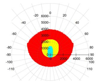
Figure 6. Performance-based safety volume for DAA (detect-and-avoid).
