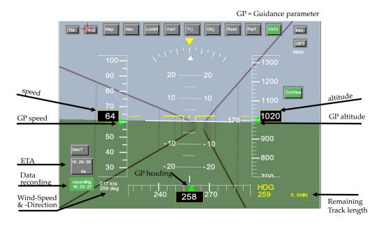
Figure 2. Tunnel-in-the-sky display (dark purple lines) and overlaid Bug-PFD-guidance display.
