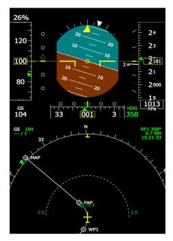
Figure 3. Primary flight display with course deviation indicator.
