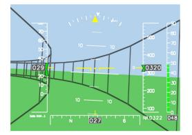
Figure 10. Highway-in-the sky concept as navigation assistance for minimally trained pilots [46].
