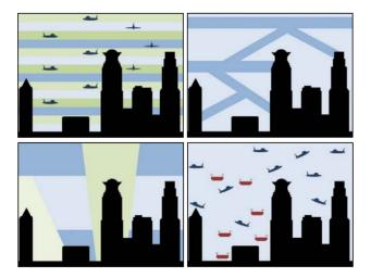
Figure 11. Metropolis airspace concepts Layers, Tubes, Zones and Full Mix [50].
