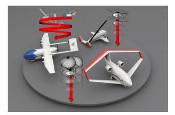
Figure 7. Possible configurations for a large cargo drone.
