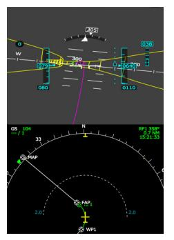
Figure 4. Synthetic vision system with tunnel-in-the-sky display.
