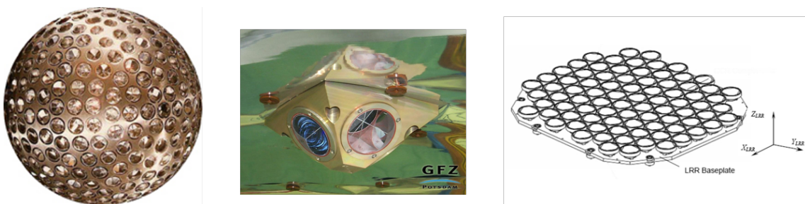
Figure 2.4: Examples of utilised CCR arrays in SLR. Left: Lageos-1, middle: Champ, right: Galileo-1. Images taken from ILRS webpage [20].
