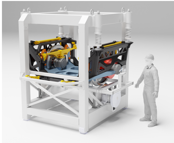
Figure 1.1: Full scale prototype and integration test rig of a running gear with IRW. Primary wheel carrier is shown in blue and secondary suspension frame is shown in black [Deu22b].
