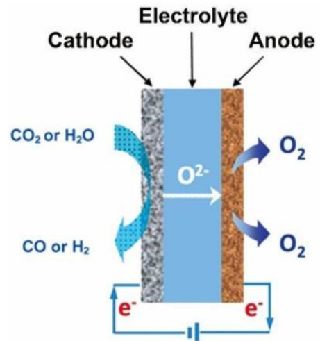
Figure 11: A typical schematic of SOEC [142]
