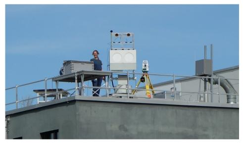
**Figure 2.** Photo of the elevated measurement set up located on the top of a building. The VNA is placed in a temperature-controlled box on the left on a table with its antennas (orange radoms) on top of the transponder (white and gray box on a positioner unit). The geodetic total station is placed on a wooden tripod right of the transponder.
