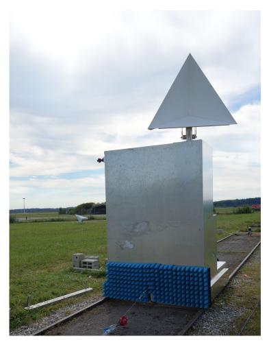
Figure 4. Measurement setup of the railway cart including absorbing material to reduce its backscatter.
