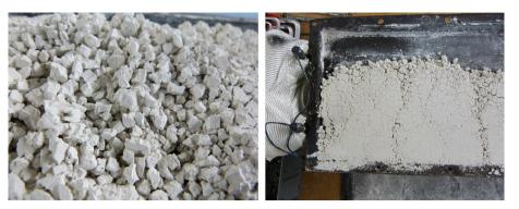
Fig. 10. Right: reaction bed after 35 cycles; left: larger agglomerates after loosening of the bed.
