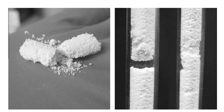
Fig. 11. Agglomerates, bridges and channels in the cycled calcium chloride reaction bed.
