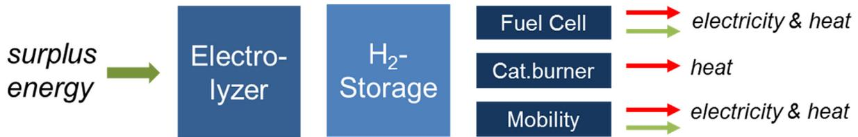
Fig. 1. Scheme of a hydrogen-based power2gas system to store surplus electrical power.
