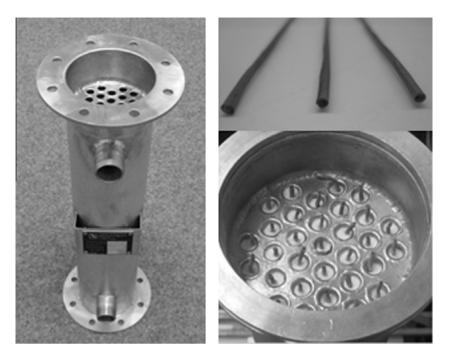
Fig. 2. Tube bundle heat exchanger, used as reactor (left) and its modification with fixed gas channels made of thin wire mesh (right).
