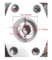
Figure 19: Combination reactor for hydrogen storage with internal preheater; left: schematic preheating process (orange area: high reactivity of metal hydride, blue area: high reactivity of complex hydride); right: picture of lab-scale reactor for model validation [Bue\_2014a]. (Further details can be found in the original publication attached in Chapter 6.)
