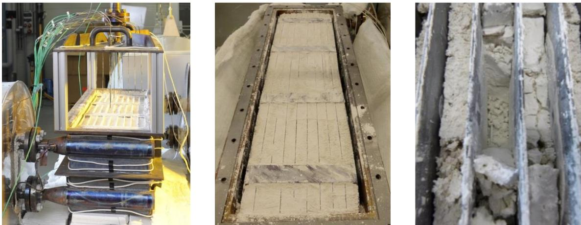
Figure 26: Plate heat exchanger for thermochemical energy storage based on  $\text{Ca}(\text{OH})_2$  in 10 kW scale; left: integration and instrumentation with opened lid; middle: material as supplied [79]; right: material after 10 cycles [78]
