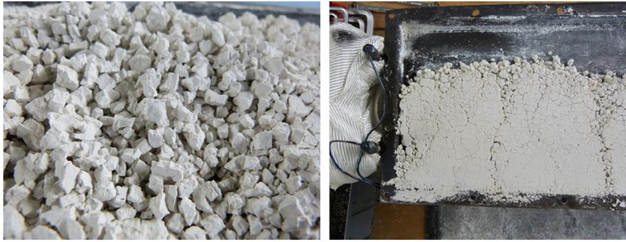
Fig. 10. Right: reaction bed after 35 cycles; left: larger agglomerates after loosening of the bed.
