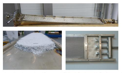
Fig. 2. Top: heat exchanger plate used as reactor; bottom left: storage material filled into the frame; bottom right: filter plate to encase the reaction bed.
