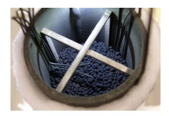
Figure 15: Lab-scale system for open thermochemical energy storage using Oxygen as reactant. Left: Lab-scale test-bench for investigation of gas-solid reaction based on oxygen; right: view into fixed bed reactor containing reactive granules of (Mn<sub>0.75</sub>Fe<sub>0.25</sub>)<sub>3</sub>O<sub>4</sub> [Wok\_2017<sup>7</sup>].
