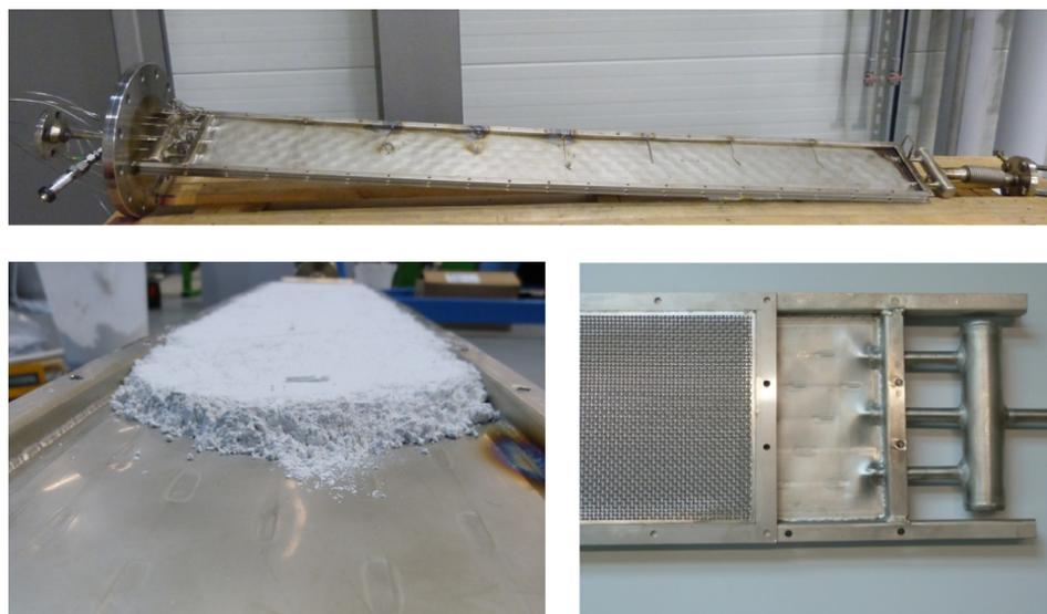
Fig. 2. Top: heat exchanger plate used as reactor; bottom left: storage material filled into the frame; bottom right: filter plate to encase the reaction bed.
