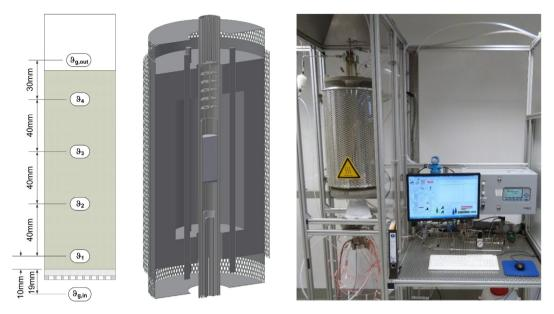
**Fig. 2.** Geometry of the reaction chamber with locations of thermocouples in the packed bed of metal oxide (left); position of the packed bed storage reactor integrated in a tube furnace with additional gas/air heater below the bed (middle); experimental setup of the test rig (right).
