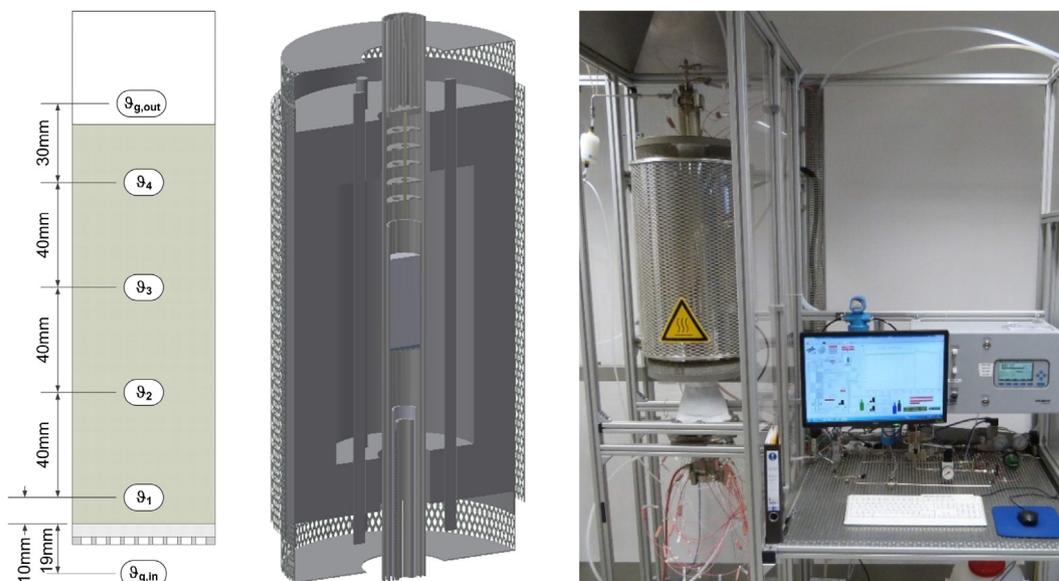
**Fig. 2.** Geometry of the reaction chamber with locations of thermocouples in the packed bed of metal oxide (left); position of the packed bed storage reactor integrated in a tube furnace with additional gas/air heater below the bed (middle); experimental setup of the test rig (right).
