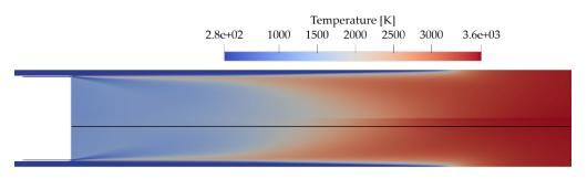
**Figure 9.** Temperature in the combustion chamber: (top) base—no pollution (rotated with symmetry axis at the top and wall at the bottom), (bottom) All-F pollution.
