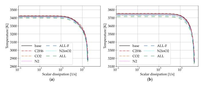
**Figure 4.** Temperature over scalar dissipation at the respective stoichiometric point (ROF = 4) for different pollutions of the fuel and/or oxidizer at: (a) 2 MPa and (b) 20 MPa.
