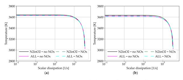
**Figure 5.** Temperature over scalar dissipation at the respective stoichiometric point comparing the influence of NOx chemistry at 10 MPa for different pollutions: (**a**) on the fuel side (N2 and ALL-F) and (**b**) pollution of the oxygen and both media ( $N_{2in}O_2$  and ALL).
