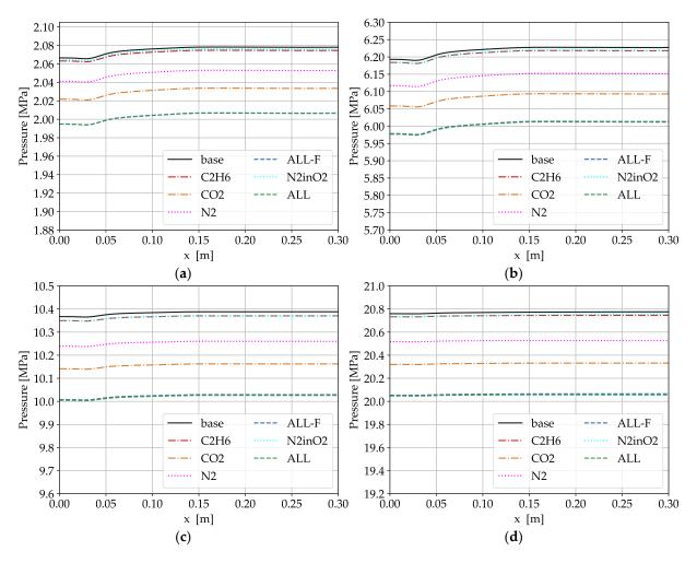
**Figure 10.** Combustion chamber wall pressure for different pollutants of the fuel and/or oxidizer at the combustion chamber configuration: (**a**) p02 (target pressure 2 MPa), (**b**) p06 (target pressure 6 MPa), (**c**) p10 (target pressure 10 MPa), and (**d**) p20 (target pressure 20 MPa).
