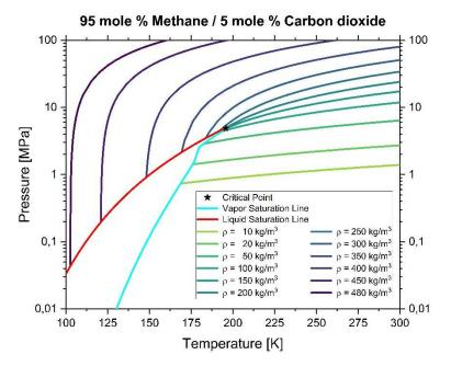
**Figure 2.** Calculated phase diagram of 95 mole % methane / 5 mole % carbon dioxide for pressures between 0.01 and 100 MPa and temperatures between 100 and 300 K. (Linear temperature scale, logarithmic pressure scale. Vapor saturation line: cyan blue color; liquid saturation line: red color; black star: critical point, densities: other colored lines).
