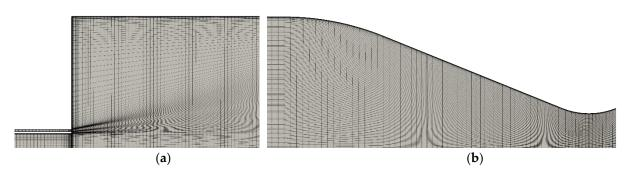
Figure 6. Numerical mesh for the CFD simulation: (a) inlet and (b) nozzle.
