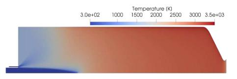
**Figure 7.** Temperature within the combustion chamber for Test Case  $C_2H_6/p06$ .
