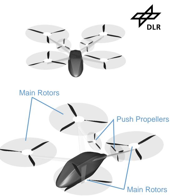
Initially developed as Medical Personnel Deployment Vehicle (Project Urban Rescue) and adapted as an air taxi vehicle for HorizonUAM.
