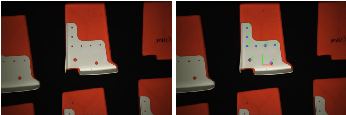
Figure 2: Image of clip (left) and the least squares fit results (right)
