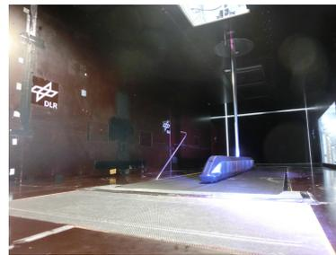
**Fig. 2:** The figure shows the NGT model inside the wind-tunnel.
