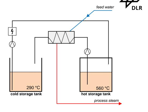
■ State of the art 2-Tank molten salt storages: 400 kJ/kg | 195 kWh/m³
