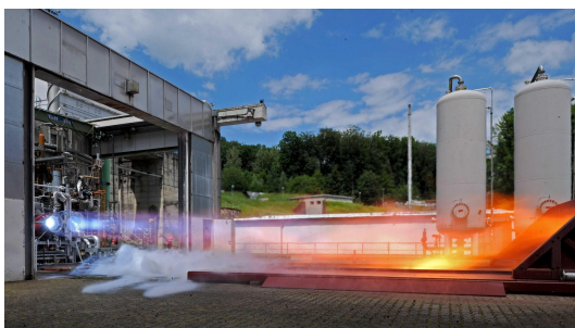
(A) ESA LOX/CH 4 demonstration engine test
