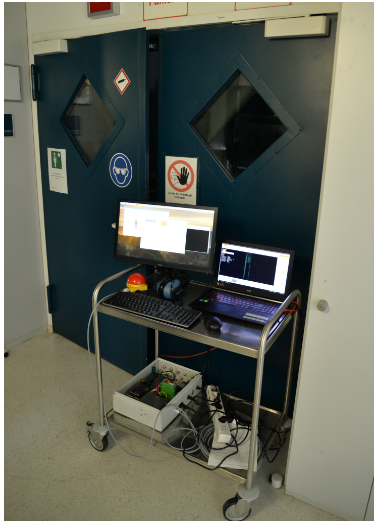
Figure 4.5: Experimental setup in the hallway outside the laboratory. The PLC is located on the lower rack and is connected to the monitor, mouse and keyboard on the tabletop. The laptop running the HS camera viewing program is also placed on the here. Red emergency stop button to quickly abort a test run if necessary.
