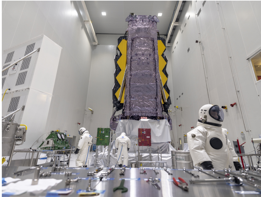
Figure 1.3: James Webb Space Telescope during fueling operations prior to launch at Europe's Spaceport in French Guiana [6].
