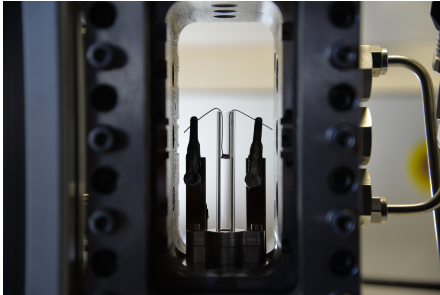
Figure 4.3: Image of the fully assembled strand plug after it has been inserted into the combustion chamber.
