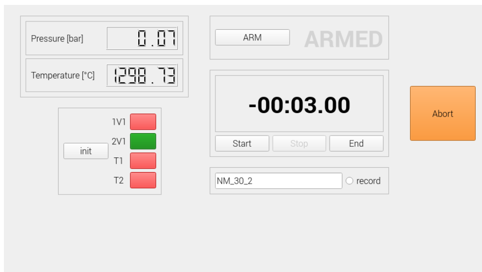
Figure 3.7: Screenshot of the controller GUI. All output signals (triggers and valves) are in their initial state and the system is unarmed.
